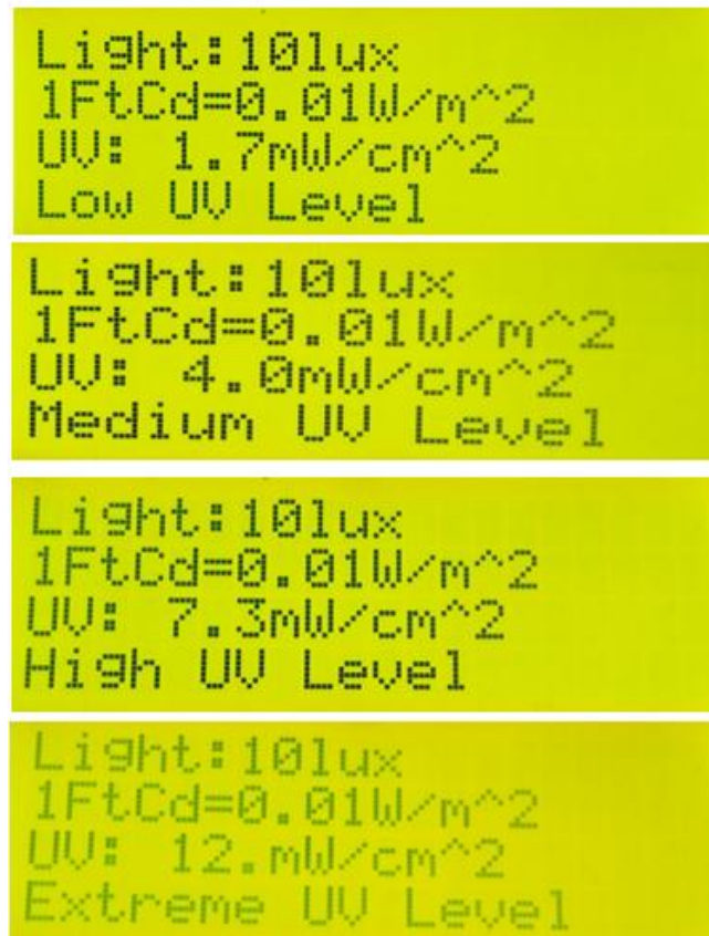
Figure 9 Testing UV index and light intensity
